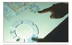
Figure 3. Dual-finger selection on multitouch tabletop display. The user manipulates the pointer with the right hand while adjusting the control-display ratio with the left.
