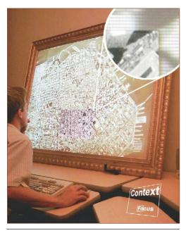
Figure 1. Focus-plus-context screen prototype. Content panned into the focus region is viewed in higher detail, making the focus display behave like a magic high-res lens.
