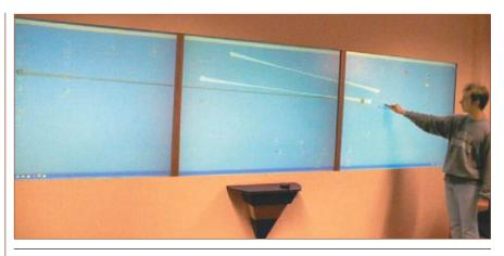
Figure 2. Drag-and-pop technique. As the user drags an icon from the right panel to the center, potential target folders "stretch" toward him, enabling him to file the icon with a small hand movement.
